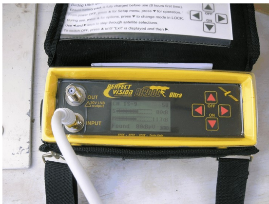
Photo of the Birdog, which is a satellite finder and signal meter we used as part of a test installation. While not strictly necessary for deployments, it is certainly a lot handier than attempting to find a signal with the dish attached to your DVB-S receiver using the receiver software on your computer to test for a lock.
